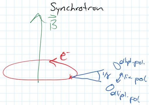
In synchrotron, rad'n is strongly beamed in the forward moving direction, so all the polarizations are squeezed into the cone of width  $w/\gamma$ . In the center of the pulse, the pol. is linear w/ an orientation normal to the projected  $\vec{B}$ -field. Off center, there is some elliptical pol.
