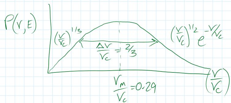
The spectrum peak occurs at  $V_m = 0.29 V_c = 1.26 \times 10^6 B \gamma^2$  (Hz)
