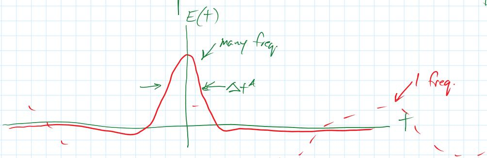
A Fourier transform of this pulse will be fairly broad b/c this pulse consists of many high freq. components
